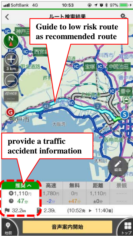
Figure 4 - The Displayed Screen of Low Accident Risk Driving Directions on Navigation Mobile
